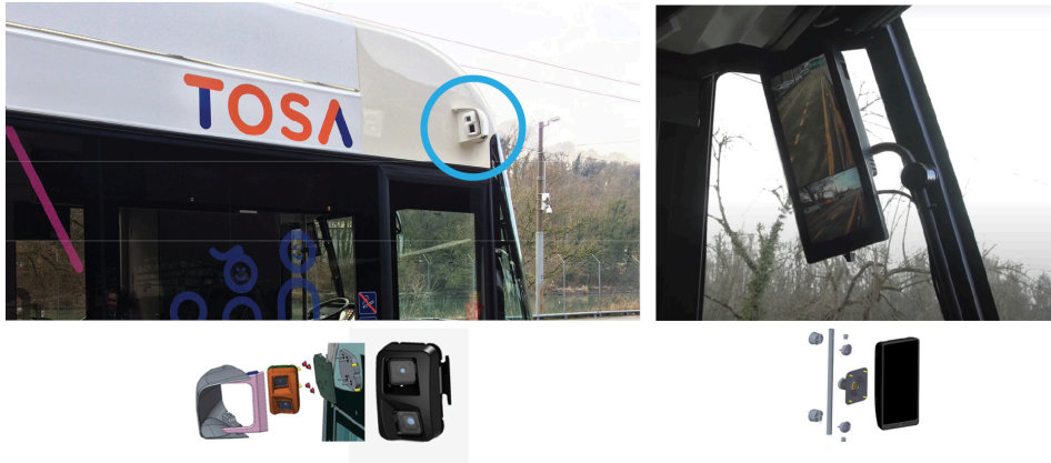
Camera affixed to exterior of vehicle; component & installation
